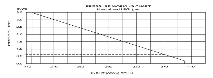
Any change from zero (0) pressure in the combustion zone will affect the Btu output of the burner. To supply the required input to the appliance, manifold pressure will have to be adjusted to compensate for this condition.
